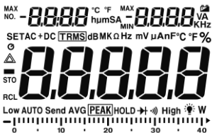
Illustration 2. LCD display of the CMM-40 meter
